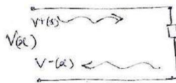
Reflection Coefficient  $\Gamma(x)$  is defined as ratio of reflected wave phasor to incident wave phasor.
