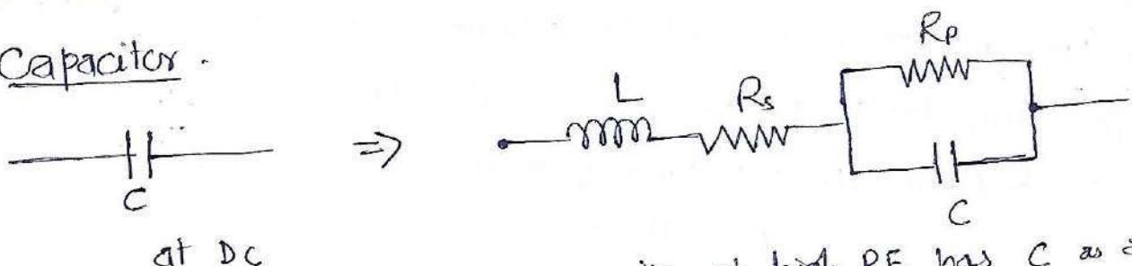
The equivalent circuit of capacitor at high RF has  $C$  as actual capacitor,  $L$  is lead inductance,  $R_s$  is the series resistance &  $R_p$  is the insulation resistance.
