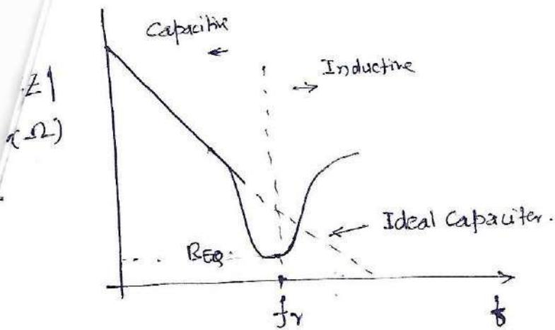
1. for  $f < f_r$  - In this region as frequency increases, the lead inductance's reactance goes up gradually, cancelling the capacitor's reactance & thus causing resonance ( $f_r$ )
