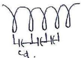
1. for  $f < f_r$ , In this region, the inductor's reactance ( $X_L = \omega L$ ) increases as freq. is increased.
