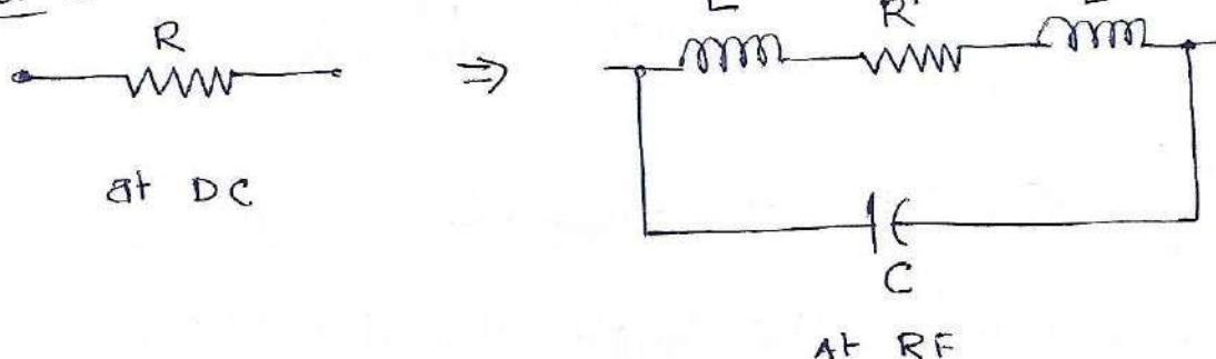
Fig. shows a simple resistor at DC. As frequency increases, the lead wire inductance ( $L$ ), increased resistor value ( $R' \gg R$ ) due to skin effect & parasitic capacitance becomes predominant, as shown in figure. The net effect of all these parasitic elements on the average, is a decrease in the resistance value of the resistor.
