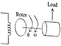
construction is similar to 2-\$\phi\$ induction motor
