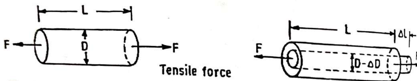
Fig. Change in dimensions of a strain gauge element when subjected to a tensile force.
