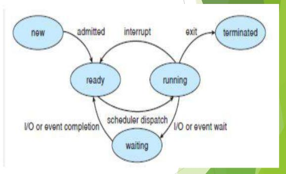
During the execution of an application program, individual tasks are continuously changing from one state to another. However, only one task is in the running mode (i.e. given CPU control) at any point of the execution
