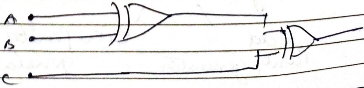
Odd Parity generator :- It maintains the Binary data's no. of 1's
